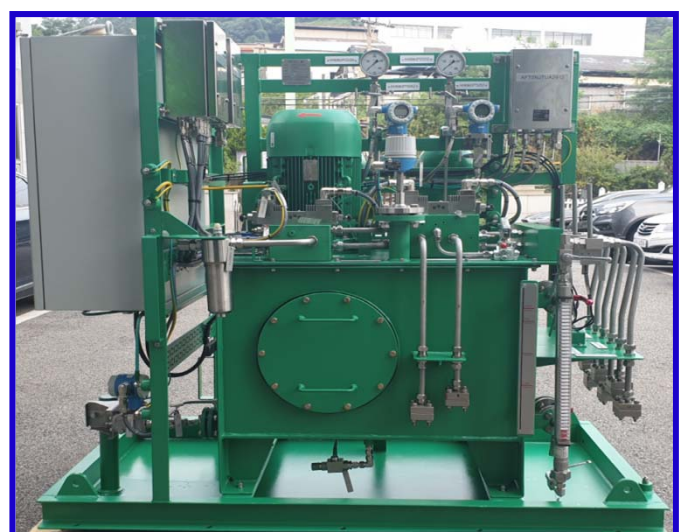
HYDRAULIC POWER UNIT FOR FPSO
