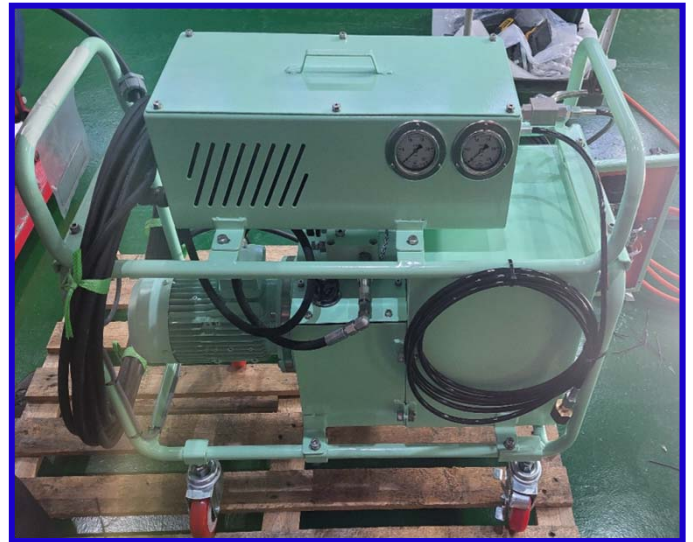
N2 CHARGING UNIT FOR SHIP YARD
