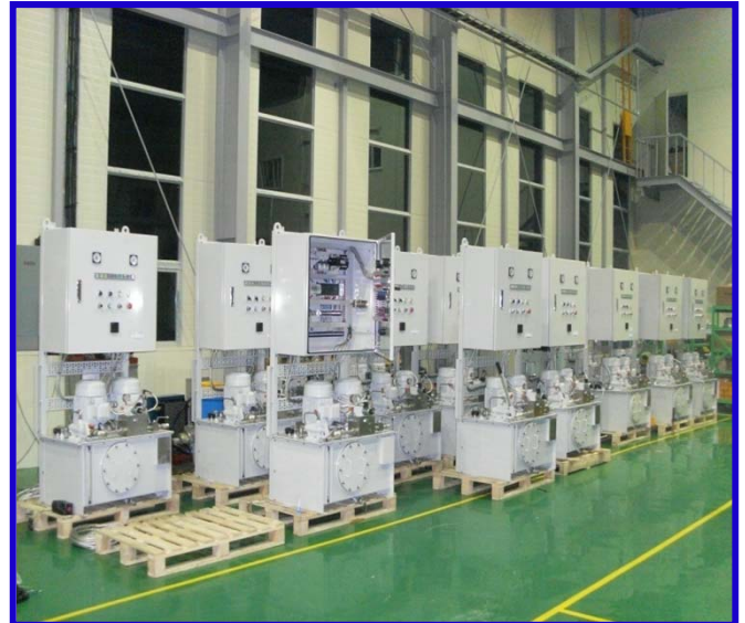
MAIN VALVE CONTROL HYDRAULIC POWER UNIT
